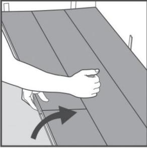
First, separate the entire row by carefully lifting it until the long joints release.
