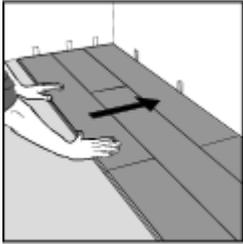
9. After 2-3 rows. Adjust, if needs be the distance between the front wall or skirting and the flooring edge and ensure adequate numbers **of 6mm spacers** are in place to keep the flooring edge a minimum 6mm away from the wall or skirting at all points along this edge.
