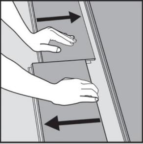
Second, **Slide the short joints** of the board to be removed **horizontally in opposite directions**. **DO NOT** lift the end of a board to separate it as this will damage the end joint.
