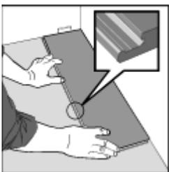
1. First board, first row. Place 6mm expansion gap spacers against the walls or skirting boards at the left hand end, and back long edge, of the first board and position the board end against the wall. The tongue on the back edge of the board should be against the spacers on the facing wall.
