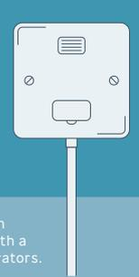
Electrical connection should be via an unswitched fixed wiring connector with a 5 amp fuse for Domestic range macerators. Professional range may vary - check individual instruction manual.
