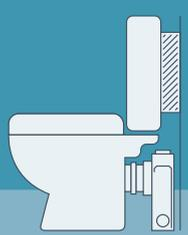
Since many closed coupled WC suites do not have the space between the WC pan spigot and the wall, you may have to batten the cistern off the wall to make room for the Saniflo. However Sanislim will fit behind most closed coupled WC suites without the need for this.
