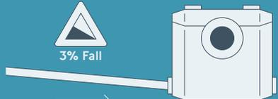
Pipes entering the Saniflo should have a gravity fall of 3%.
