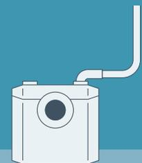
If a vertical lift is needed, this should be as close to the start of the run as is practically possible and from the highest point there must be a minimum 1% fall. The closer the vertical lift is to the machine, the more efficient the pump will be.
